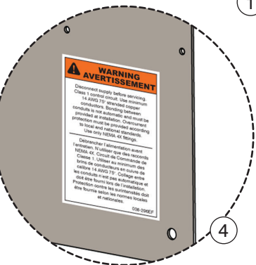
ATTACHED TO DIVIDER PLATE IN PLATINUM SERIES
