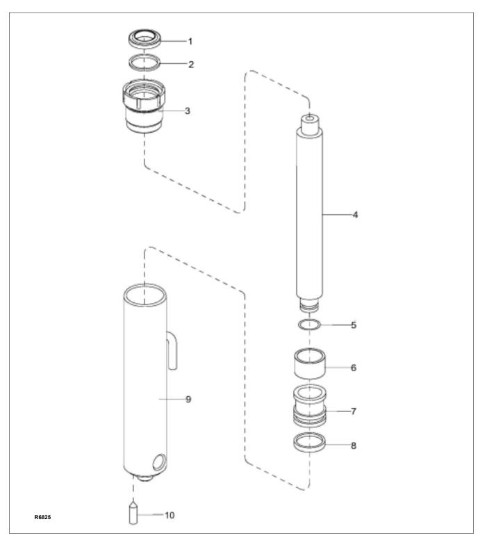
Figure 9-3 Lift Cylinder (Telescopic)
