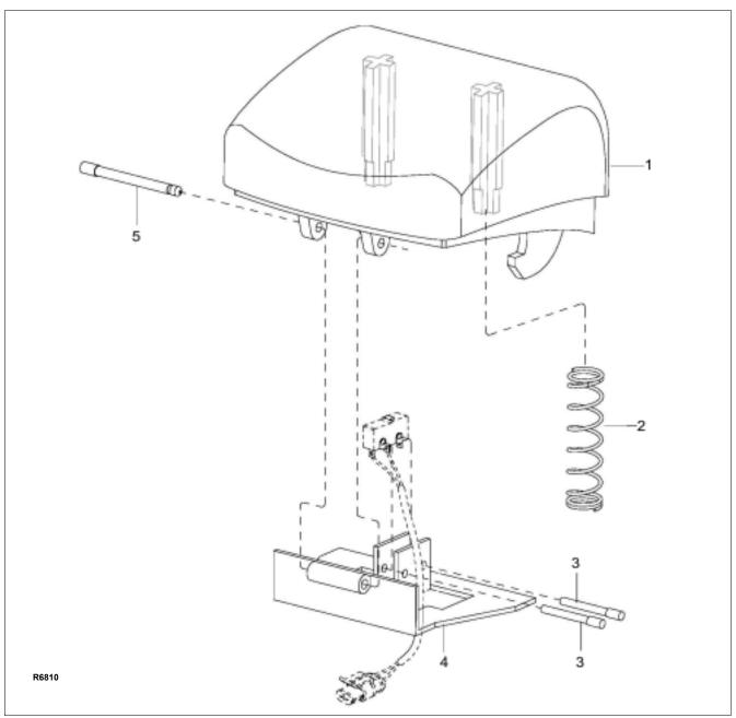
Figure 5-3 Emergency Reverse Switch Assembly
