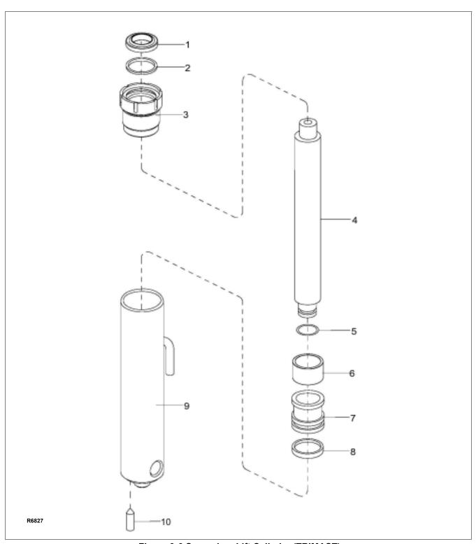
Figure 9-6 Secondary Lift Cylinder (TRIMAST)
