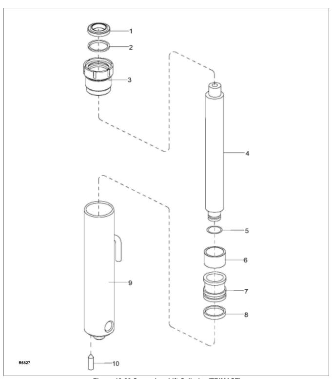
Figure 12-23 Secondary Lift Cylinder (TRIMAST)
