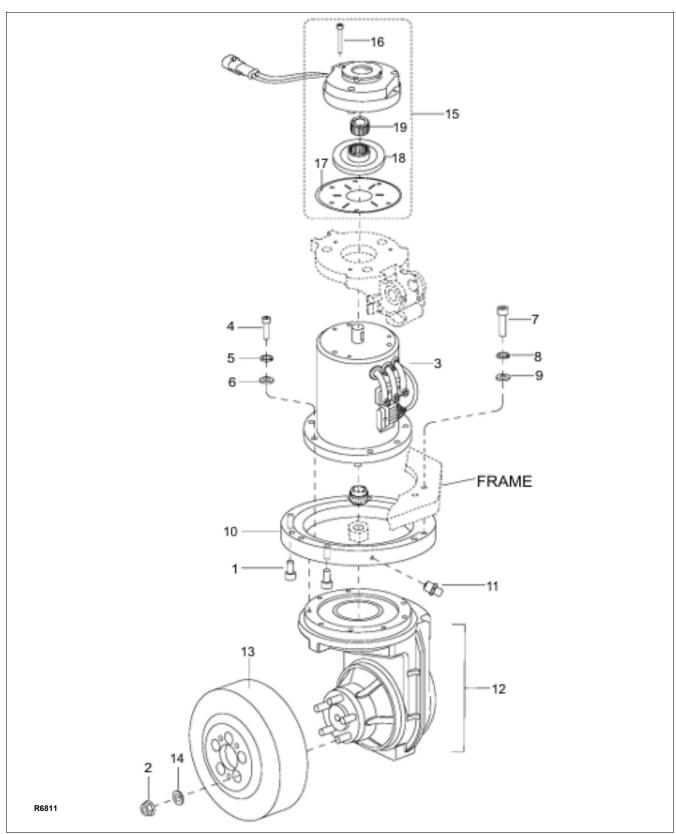
Figure 10-3 Transmission, Motor, Brake Assembly
