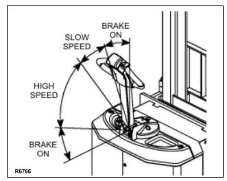
Figure 2-5. Brake Actuation
