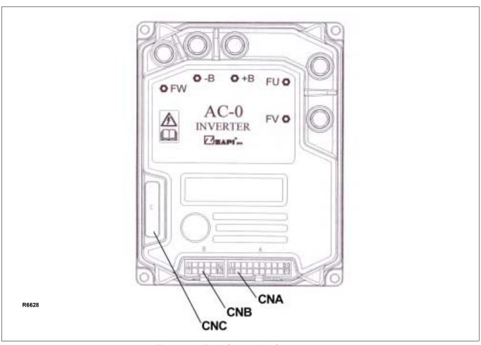
Figure 4-6 Zapi Controller Connectors
