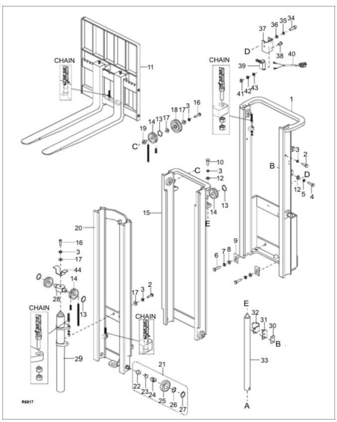
Figure 12-12 Elevation System (TRIMAST)
