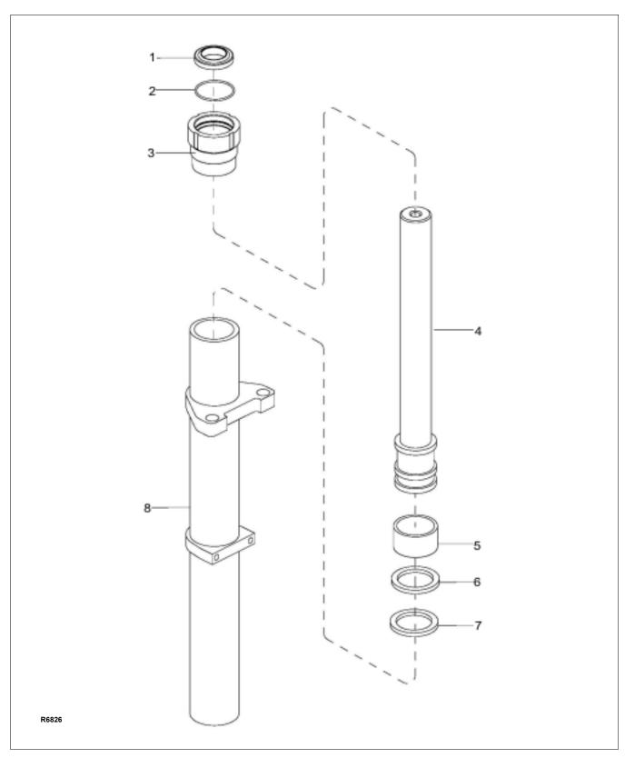
Figure 12-22 Free Lift Cylinder (TRIMAST)
