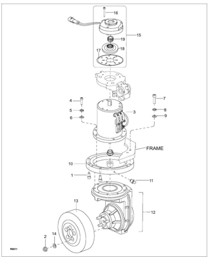
Figure 7-1 Transmission, Motor, Brake Assembly
