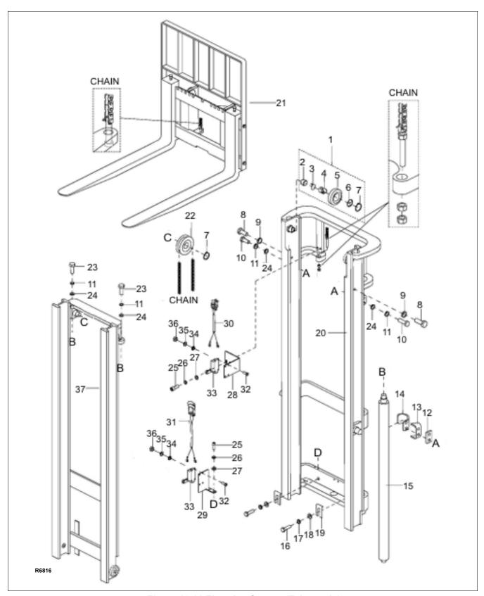
Figure 12-11 Elevation System (Telescopic)
