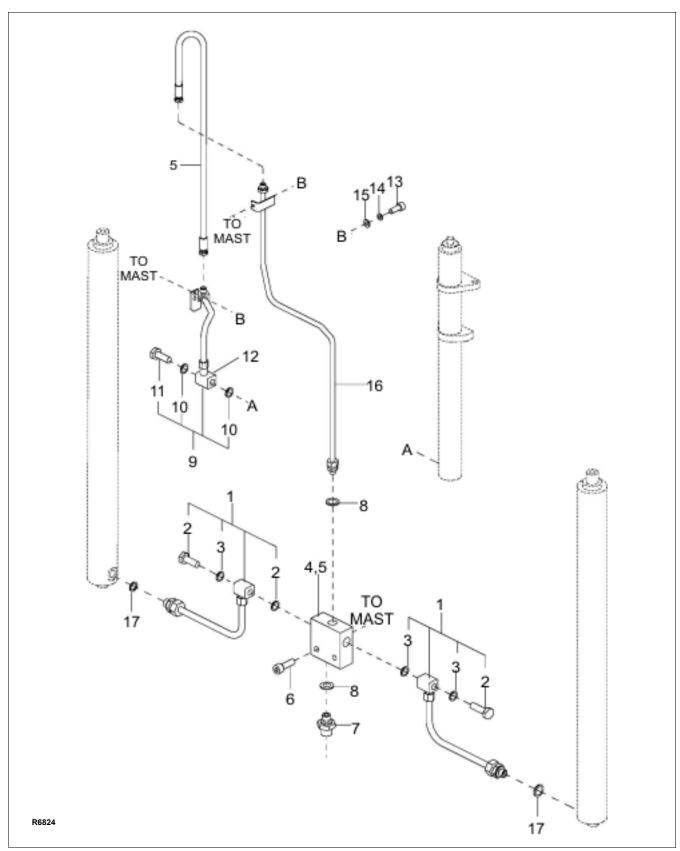
Figure 12-20 Hydraulic System (TRIMAST)
