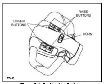
Figure 2-4. Pushbutton Switches
