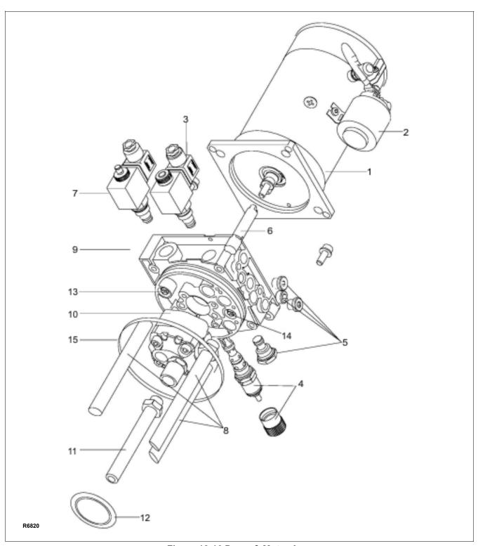
Figure 12-16 Pump & Motor Assy
