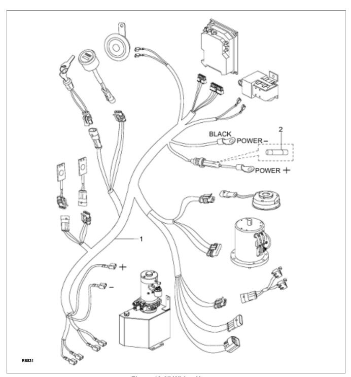
Figure 12-27 Wiring Harness
