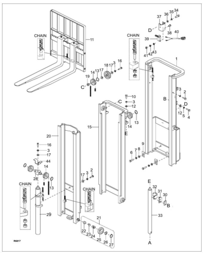
Figure 8-3 Mast (TRIMAST)
