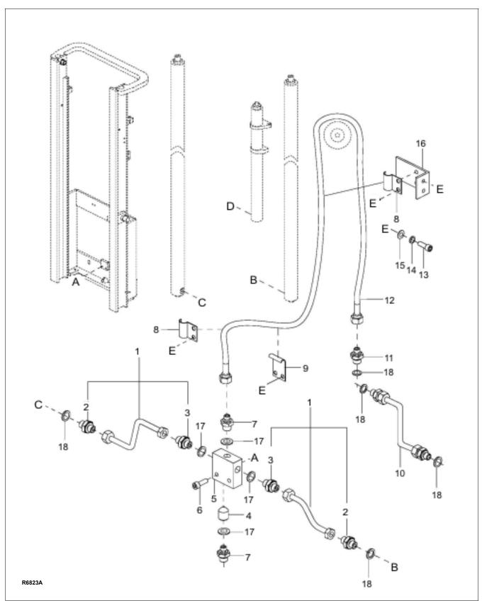
Figure 12-19 Hydraulic System (TRIMAST)
