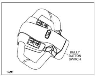
Figure 2-6. Belly-Button Switch
