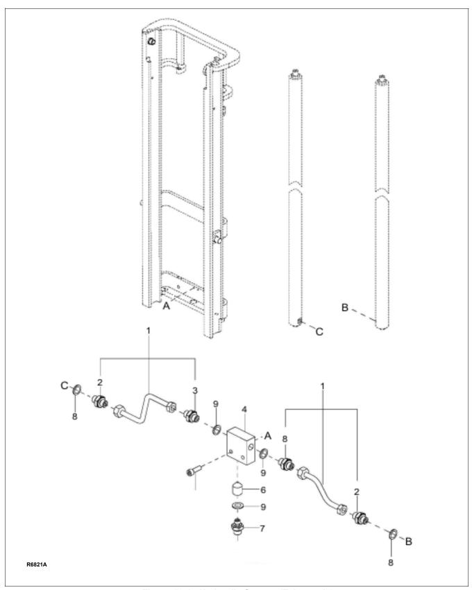
Figure 12-17 Hydraulic System (Telescopic)
