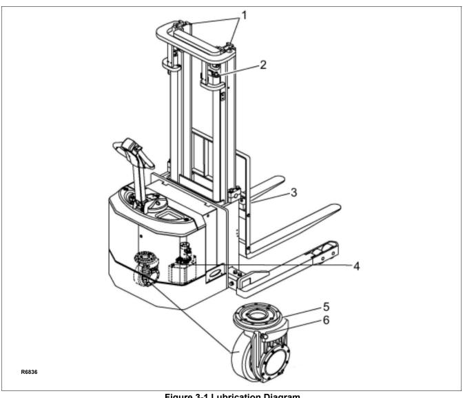
Figure 3-1 Lubrication Diagram
