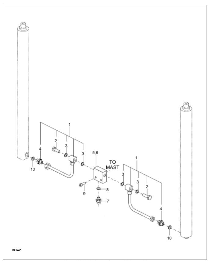
Figure 12-18 Hydraulic System (Telescopic)
