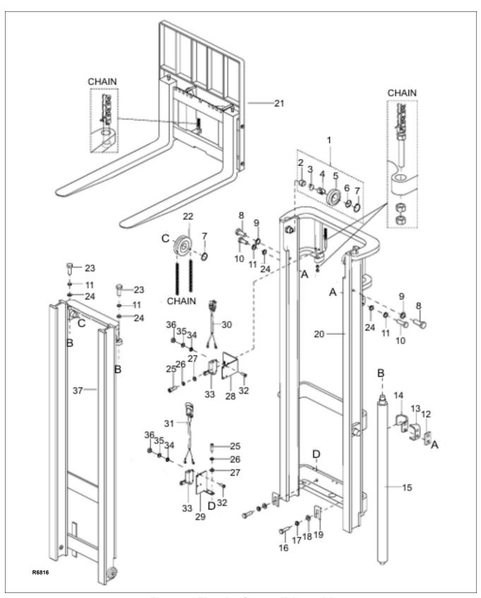
Figure 8-2 Elevation System (Telescopic)
