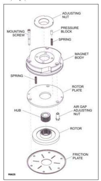
Figure 6-1 Brake Assembly
