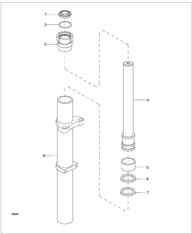
Figure 9-5Free Lift Cylinder (TRIMAST)
