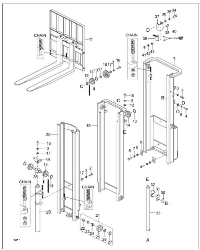
Figure 9-4 Mast (TRIMAST)
