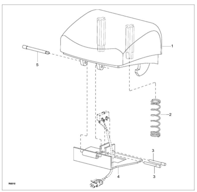
Figure 12-4 Emergency Reverse Switch Assembly
