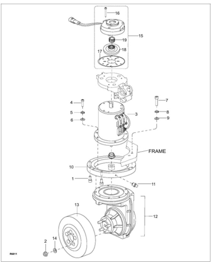
Figure 12-5 Transmission, Motor, Brake Assembly
